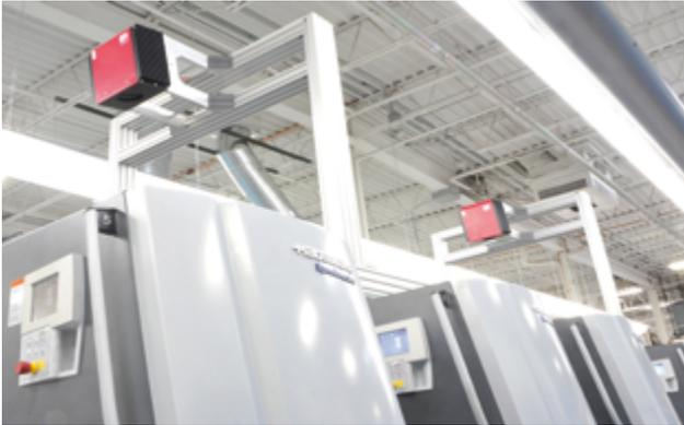
Designed for the **Heidelberg Speedmaster XL106**, the EyeC ProofRunner Sheetfed is an in-line system that **monitors the quality of leaflets on both sides during printing**. Available for both new and existing presses and less expensive than competitive systems, it offers leaflet producers a cost-effective and flexible solution to improve their print quality.
